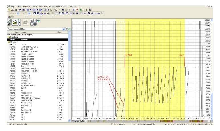
Take your best guess at the beginning and end of the map. This one has a wide bar at each end. Using your keyboard, hold down Ctrl key and press left or right direction key. You will see the grid behind the trace, move.
