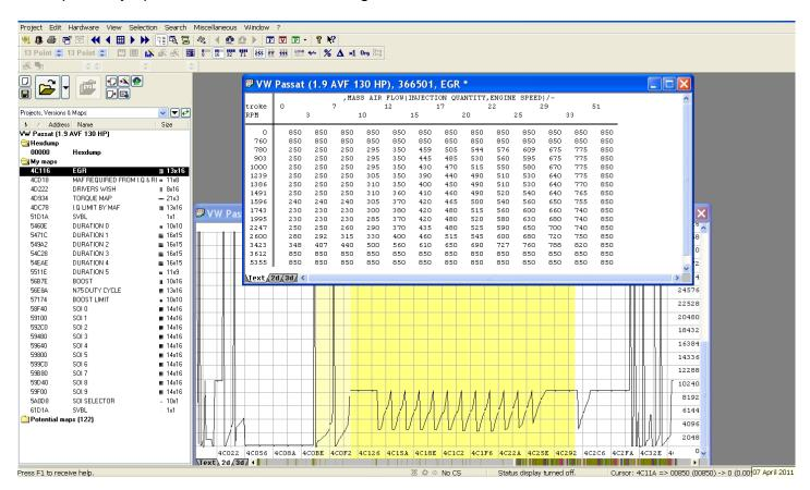
The text view numbers tell the ecu what it should be telling the EGR valve to do.
