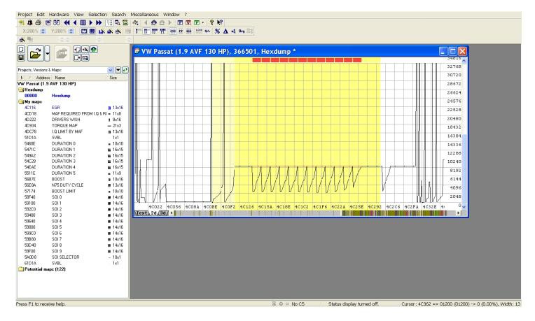
Any changes you made in the map will be automatically made in the "hexdump". AND the changes will be made using the correct values for the hexdump.
